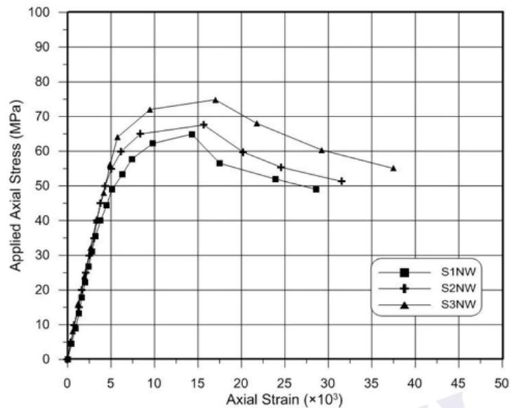
b) Axial Stress versus Axial strain for square specimens with normal concrete (NW)
