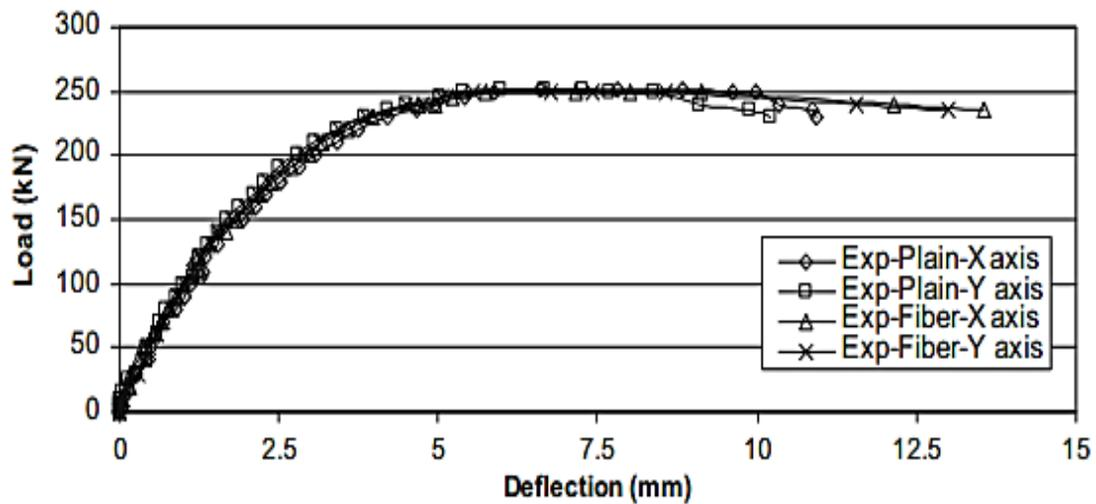
Figure 2.2 : Experimental Load-Deflection Curve for specimen size 100 mm x 100 mm x 4 mm (Tokgoz & Dundar, 2010)
