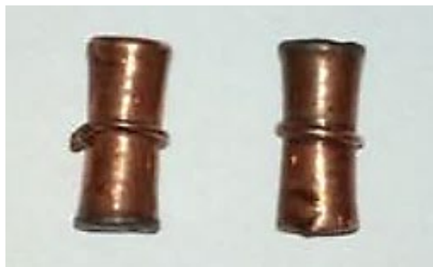
Figure 1.3: Electrode fabricated by FDM (Equbal et al. , 2017)
